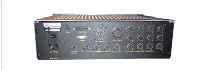
The VIPER 4120TC's rear view displays multiple input channels.
